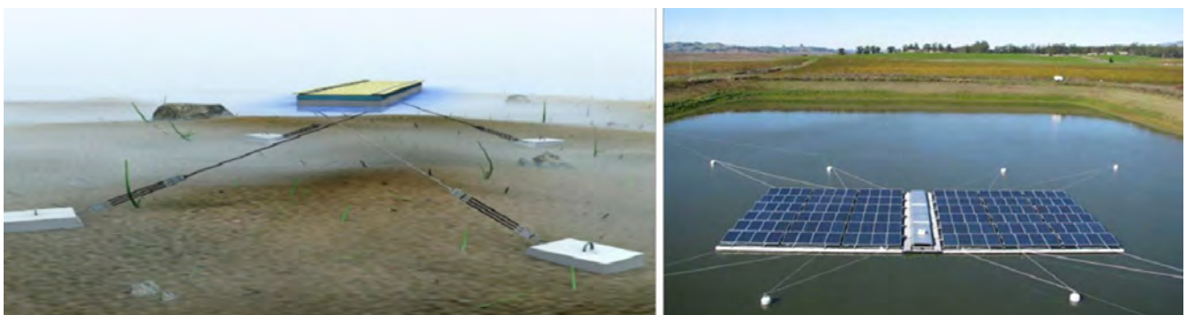
Figure 8 Illustration of Bottom Anchoring System (left) and Actual Image of Bank Anchoring System (right)
